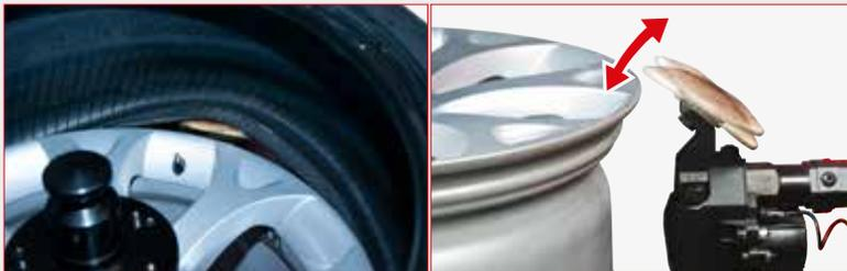
**Quick second bead demounting procedure** made possible by a **patented disc movement**, particularly useful with stiff sidewalls.
